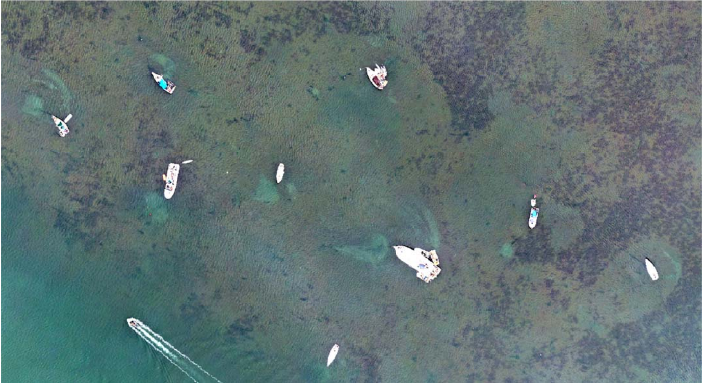
Eelgrass damage from mooring ground tackle dragging and vessel grounding drags at low tides. The dark mottling is eelgrass, the brownish tinge is a diatom film on the bottom and the bluegreen color is unvegetated silt and clay from recent disturbance. (Photograph taken June 2019)
