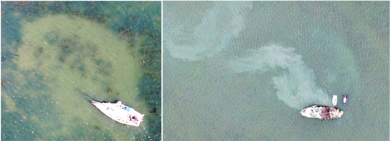
Sweep radius illustrating concentric impact areas of ground tackle on the inner portion of the sweep and keel drags on the outer portion of the sweep (left). Low tide turbidity plume generated from vessel grounding at the outer margin of the sweep radius. Note the vessel keel drag scar on the bottom above dinghies in photograph (right).
