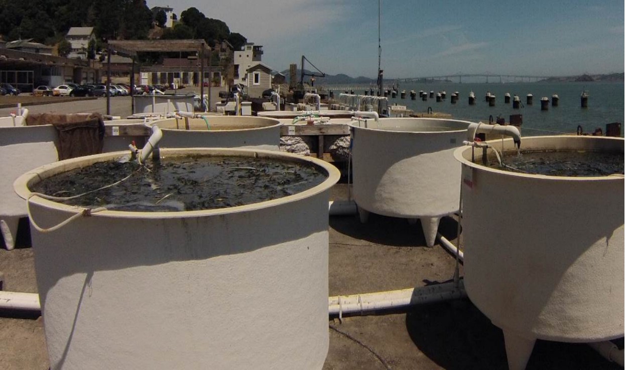
Flow-through seawater tanks used to store eelgrass from donor sites until processed into planting units. Tanks were then used to store processed planting units until they were planted at the transplant receiver sites.
